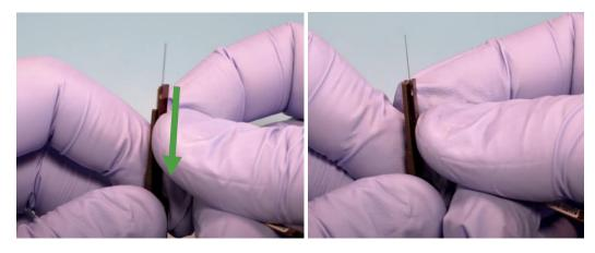
**Important note** – hold the probe in place until you tighten the screw. This will help ensure the probe does not slip out of the tweezer fingers, due to gravity, prior to securing it in place. You can lightly push on the probe dovetail to test that it is securely held by the tweezers.
