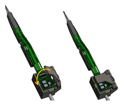
The headstage holder is secured to the probe mount shaft via a friction fit and set screw. If you need to adjust the position of the headstage clamp, you can simply loosen the setscrew, adjust the headstage position, and retighten.
