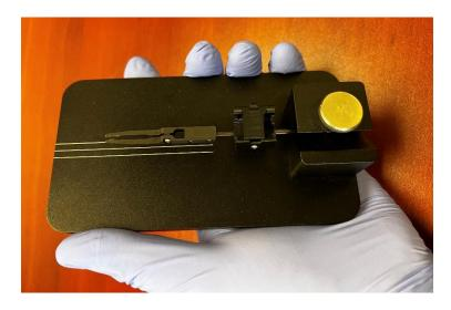
Press the dovetail flush and parallel with the NP2.0 tweezer tips, so the dovetail is in position to slide between the tweezer tips.
