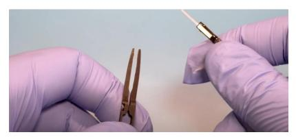
Press the dovetail flush and parallel with the NP2.0 tweezer tips, so the dovetail is in position to slide between the tweezer tips.
