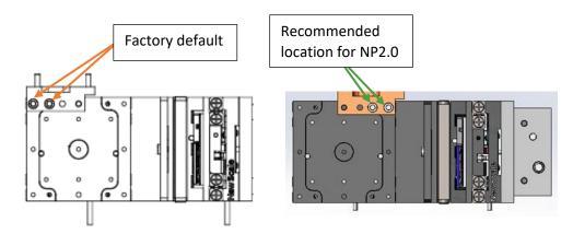
Use the included alignment pins (2) captured Philips head screw (1) to mount the MPM-Probe Mount-NP2.0 to Z-stage mount plate, as pictured below.
