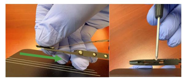
**Important note** – keep the probe horizontal, parallel to your worksurface, until you tighten the screw. This will help ensure the probe does not slip out of the tweezer fingers, due to gravity, prior to securing it in place. You can lightly push on the probe dovetail to test that it is securely held by the tweezers.
