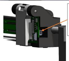
Headstage pin connector in bottom cutout, and facing down
